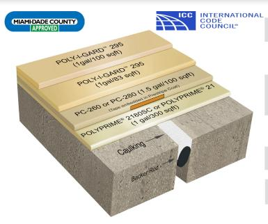
Concrete Substrate (properly prepared substrate)
